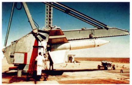
Falstaff was a British sounding rocket used during the 1970s. It used the largest solid booster ever built in the United Kingdom, the Royal Ordnance Stonechat. This motor (Stonechat Mk2) was 5.3 m (17 ft) long and 92 cm (36 in)in diameter and weighed 5090 kg with 4340 kg of propellant. It delivered an average thrust of 240 kN during 37 seconds.
